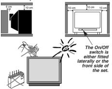
The TV set has been designed for use in dry rooms. Should you exceptionally operate it in the open air (example: on the balcony, in the veranda or tent), you must absolutely protect it against moisture (dew, rain, splash water). Prior to put up into operation a cold TV set in a warm room, you should wait until the possibly misted-up screen has dried by itself. In no case should you dismantle your TV set yourself.
